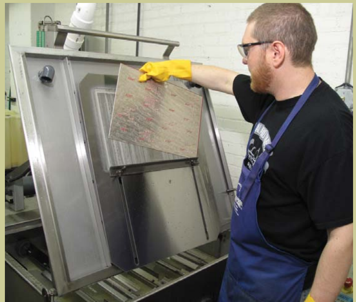
Magnesium plates for heat-stamp presses are acid-etched for label production.
