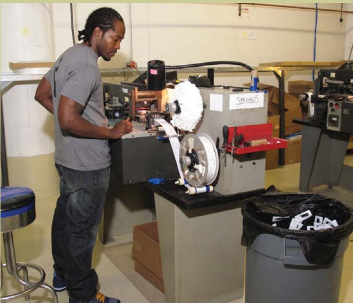
Labels for cassette projects are die-cut, printed and Brailled on National Audio's presses.
