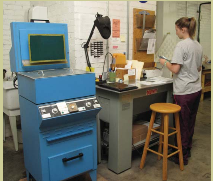
Flexible plates are produced from film for cassette imprinting.
