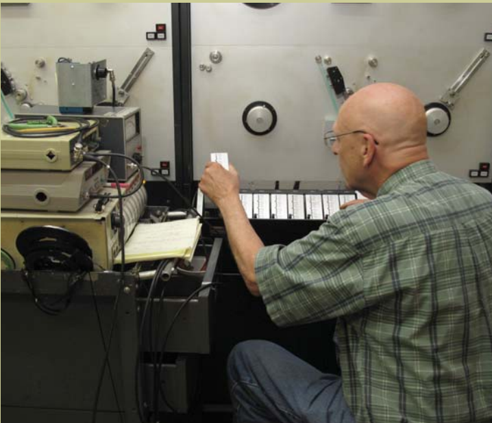
Chief Technical Engineer Bob Coverston tests Lyric duplicators for correct bias, azimuth and record levels.
